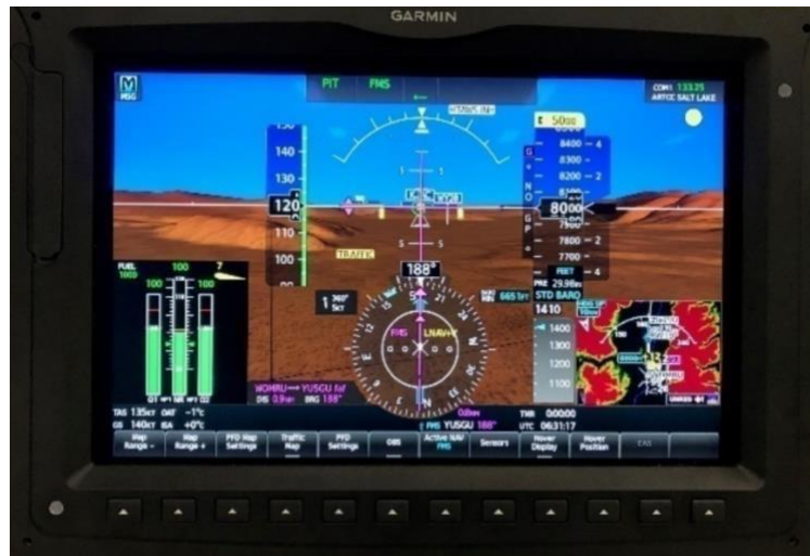
Figure 8: Garmin 12-inch 4k UHD Displays with SVT and Moving Map
