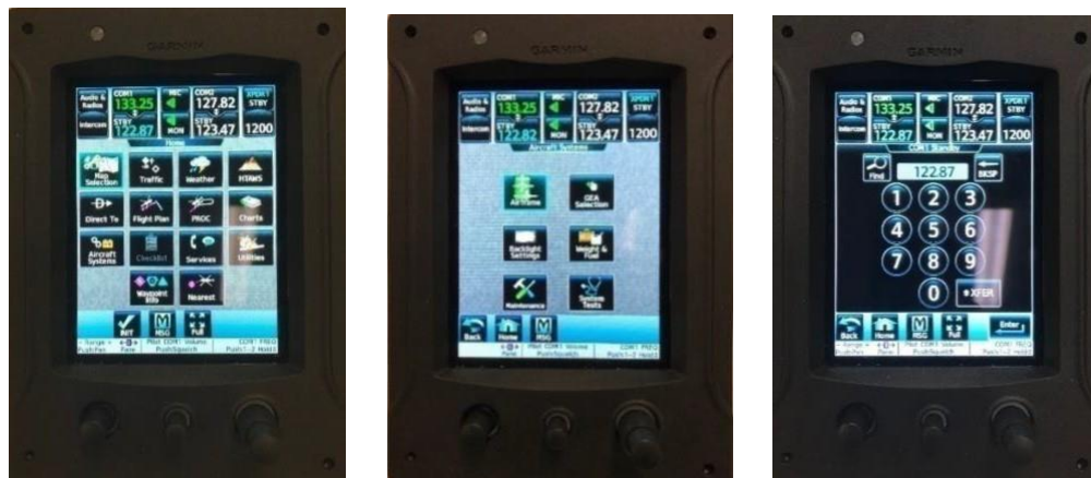
Figure 11: Garmin GTC 575H Touchscreen Controllers
