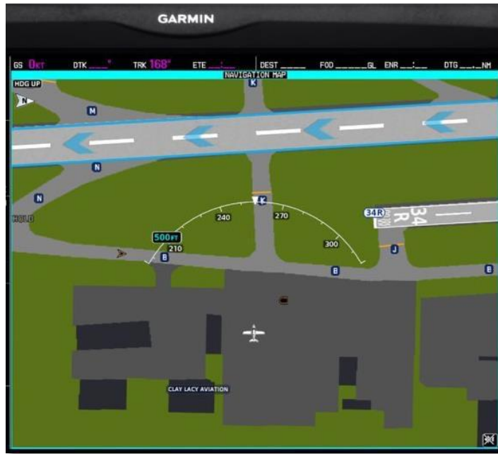
Figure 7: MFD Display of Airport Features Using SafeTaxi
