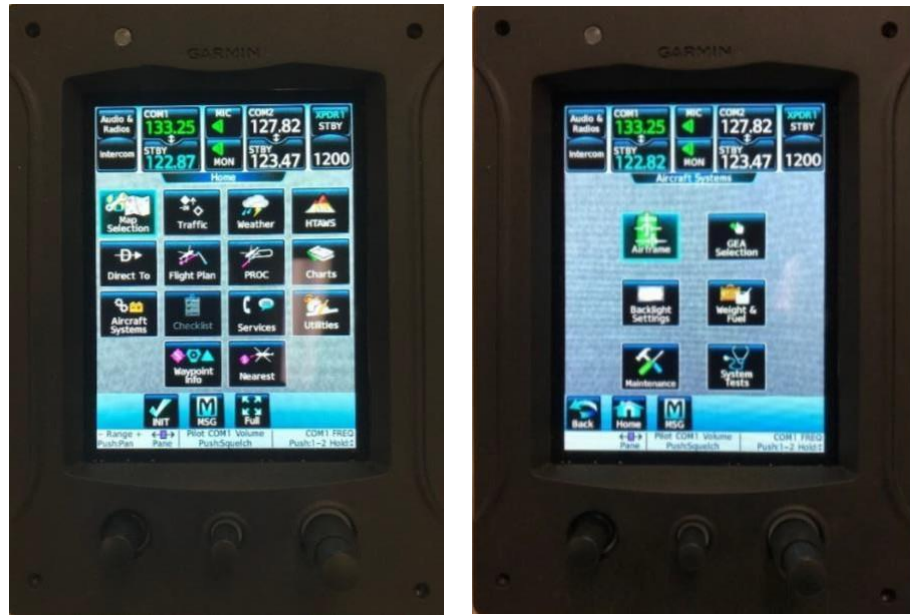
Figure 4: App-Based Garmin GTC 575H Touchscreen Controllers
