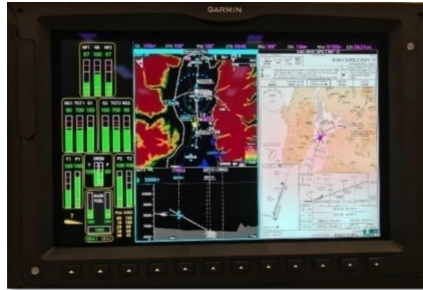
Figure 10: MFD Display of Instruments, Moving Map, and Approach Plate
