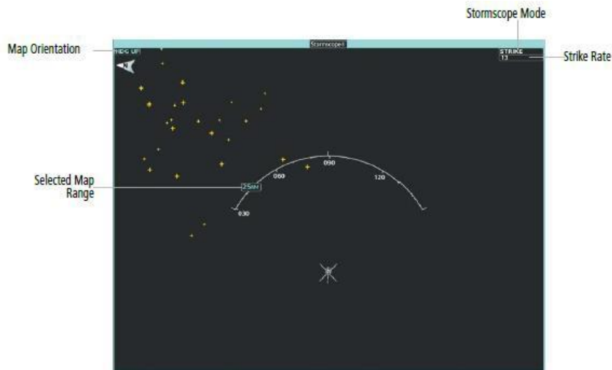
Figure 15: Stormscope Pane Operating in Strike Mode
